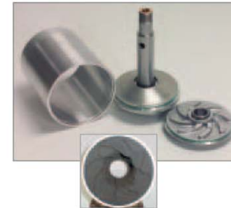
Visible proof. Clean (top) and dirty (inset) rotors from a Model 3600 centrifuge, show actual contaminants removed in one interval.
